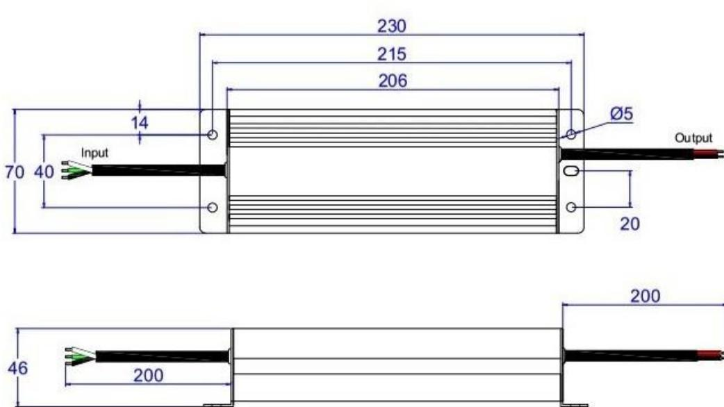
※ Input black(L) and white(N) wires to be connected AC, Green wire to be connected ground; output red and black wires to be connected led lighting.
