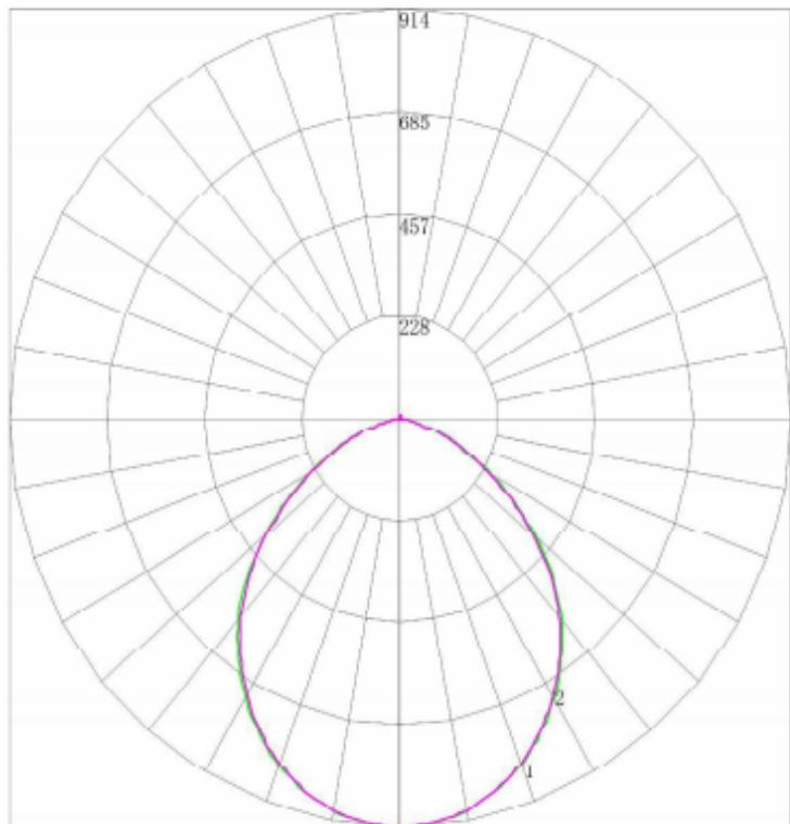
Maximum Candela = 913.9 Located At Horizontal Angle = 75, Vertical Angle = 1
